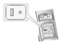
The AUX input is located in the center console.
